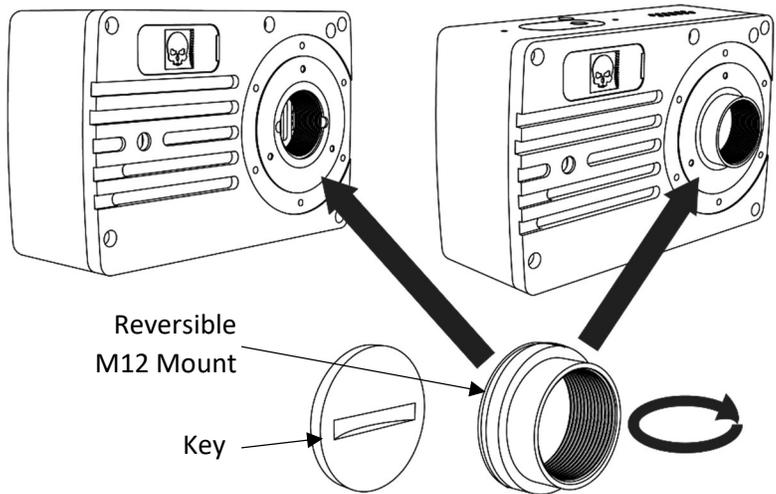
**C-Mount Lens Mounting / IR-Cut Filter**
