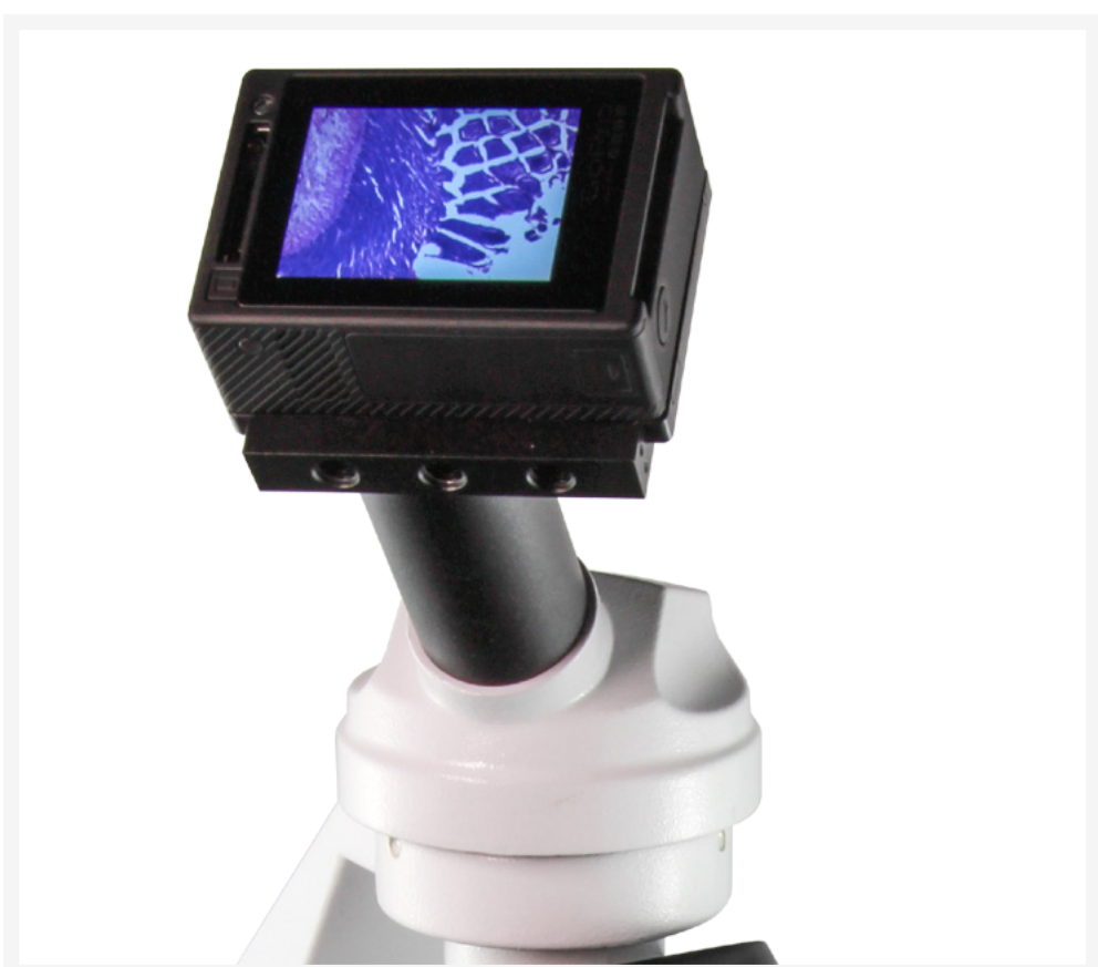
Close up look at the Ribcage modified GoPro on a standard microscope
